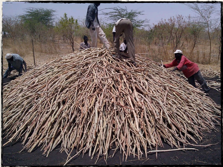
Here is our first batch of charcoal in the making utilizing the Casamance method, 30% increased efficiency.
