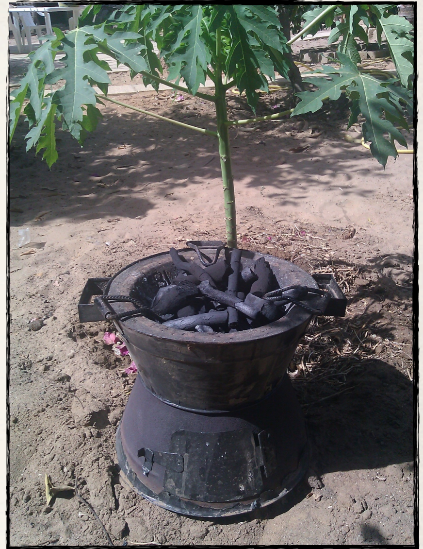
This is an example of a medium sized Jambaar stove with our charcoal. (note the thick ceramic lining that houses the charcoal) Combined savings of 65%
